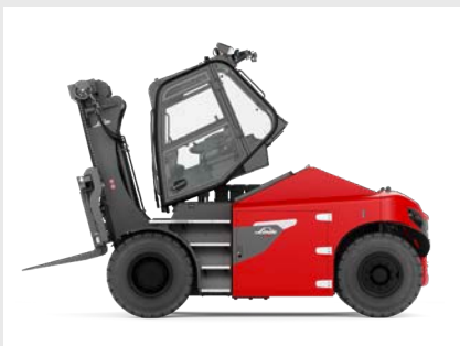
Service access through tiltable cabin
