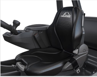
Decoupled operator's workstation
