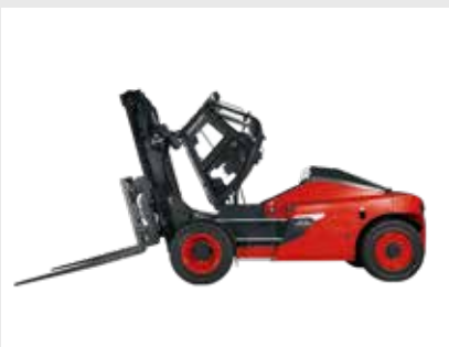
Engine access through tiltable cabin
