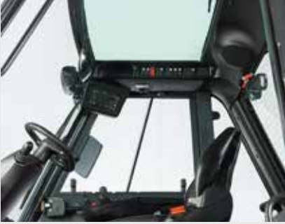
Armoured glass roof
