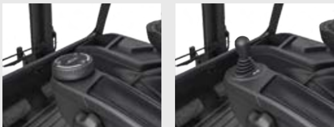
Steer-by-wire The mini-wheel (left) as the standard variant of Linde Steer Control is recommended for all the usual applications of a forklift truck: from transport over longer distances and maneuvering to storage and retrieval. The joystick (right) is particularly impressive in tight spaces.
